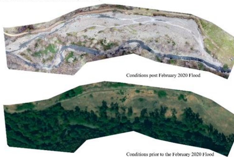
Figure 5. Expansive deposition of barren gravel and cobble substrates are common throughout the treatment area.
